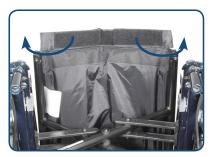
2. Pull outward on velco° strips to free them from underside of seat.
